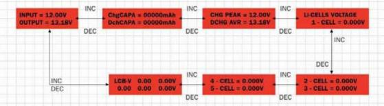
When the Battery Type button is pressed for over 3 seconds, the data view will be displayed as above.
