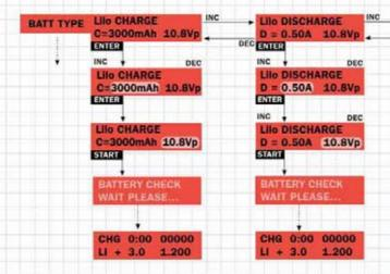
For safety purpose, this charger is designed to automatically deliver 1C charge rate to the batteries of either Li-lon or Li-Po based on user selected battery capacity.
